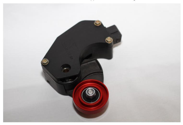
6. Check that pulley sits flush with sensor body and spins without binding. The bearing is sealed and thus will not spin for an extended time, this is normal.
