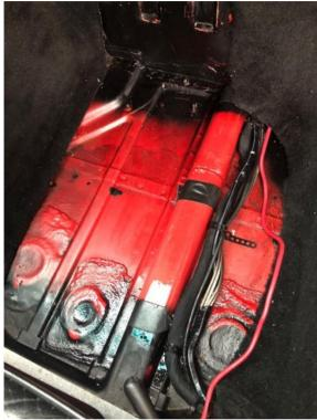
3. Install floorboard and mark center of two holes to be drilled
