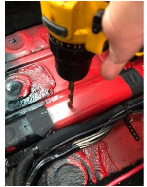
5. Install Rivnut in drilled hole
